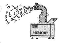
Once the data has been put in digital form, it is stored in memory. The memory must be able to store at the same rate as the A/D samples for most digital architectures. That means that if the sample rate is 200 MHz, the memory must have a write cycle time of 5 ns. Most digitizing scopes use special FISO (Fast In, Slow Out) memories for storage.
