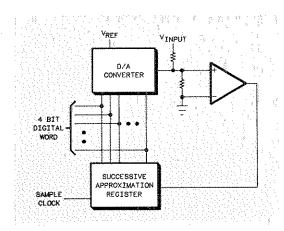
It takes N passes (where N is the number of bits of resolution) and N clocks for a successive approximation convertor to convert an analog voltage to a digital output. While this scheme provides high resolution, it is not fast enough for use in a single-shot digitizing scope. Since a repetitive digitizing scope doesn't have to sample as quickly as a single-shot one, the successive approximation A/D may be used in repetitive architectures.
