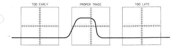
How does the trigger circuit know when to trigger? It gets a replica of the signal, called the sync pickoff, from the selected trigger source. This sync pickoff is compared to a pre-set trigger voltage that is set with the front panel trigger level knob. Most analog scopes let you specify a slope as well as a trigger voltage. This allows you to trigger at a specific point on a rising or falling transition.
